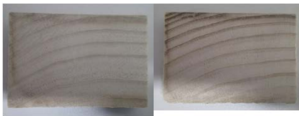
Figure 7: Condition of cross-sections of the Accoya® stake removed from the marine field trial after two years of exposure.
