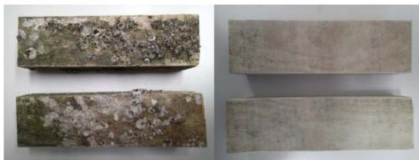
Figure 6: Condition of sections of the Accoya® stake removed from the marine field trial after two years of exposure, a) after partial cleaning of the adhering marine organisms, and b) after complete removal of the adhering marine organisms.
