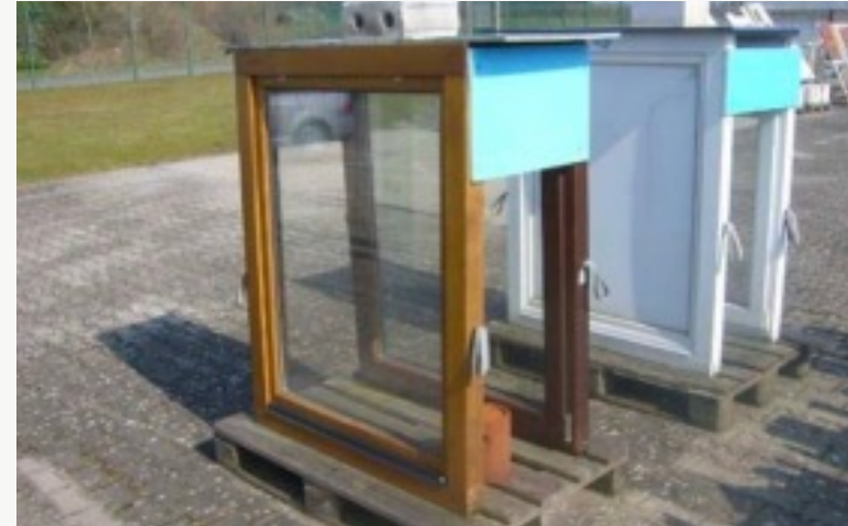
No coating degradation visible after 14 years
