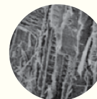
Cell structure – normal kiln dried timber
