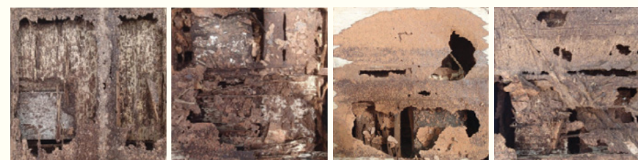
Example of attack by C. acinaciformis termites to bait-wood after 38 weeks' exposure in a Hazard Class H3 field trial.
